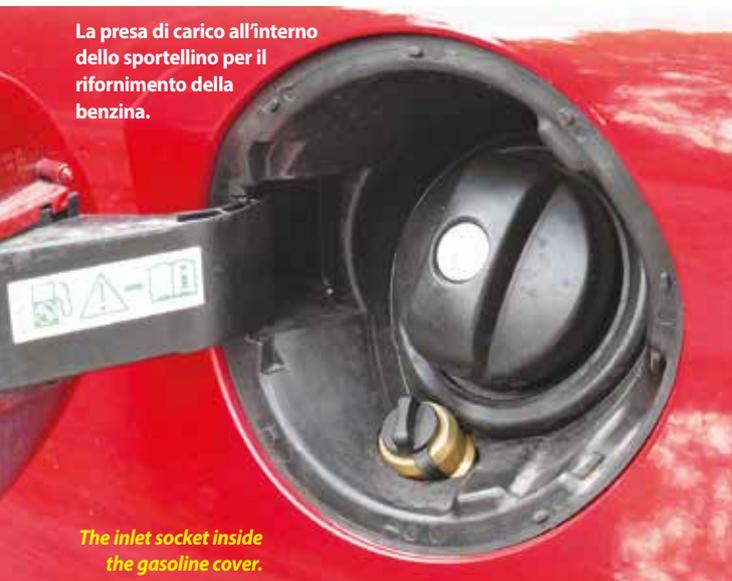
The inlet socket inside the gasoline cover.
